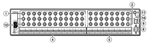
Figure 2-10 — MAV Plus 128 HDA matrix switcher
